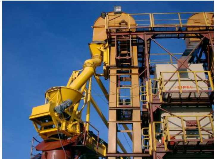
Discharge arm turret F.E.M. analysis. Design of all the mechanical gears
