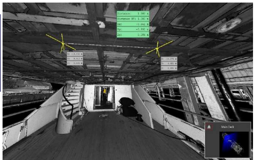
Aftend Area on Main Deck The image is NOT a photo, it shows a cloud of points obtained by 3D laser scanning. Over the points, it is possible to measure the coordinates as it is illustrated in two points.
