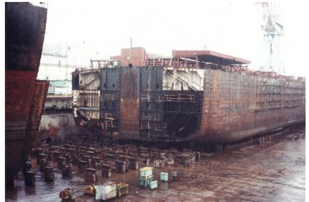
Forward section of the Alianza G1, prepared for the connection
