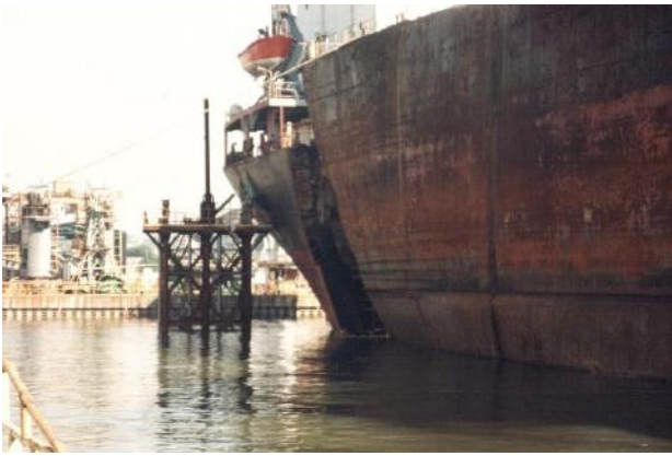
Karinas forward section afloat and ready to be removed
